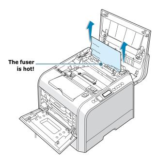
**CAUTION**: Do not touch the fuser. It is hot and could cause burns! The fuser's operating temperature is 180°C (356°F). Take care when removing paper from the printer. 6 After making sure that the left cover is open, close the top cover. Make sure that it is securely latched.
